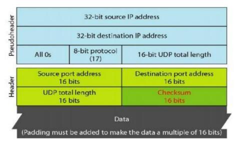
Figure 4.10 Pseudo header for checksum calculation
