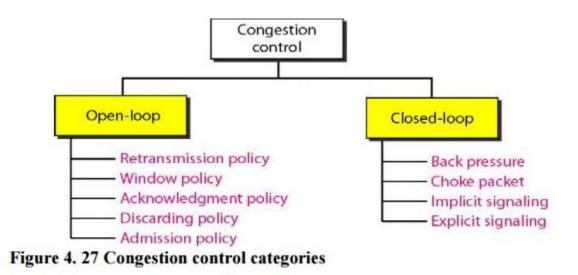
In general, we can divide congestion control mechanisms into two broad categories: open-loop congestion control (prevention) and closed-loop congestion control (removal) as shown in Figure 4.27.
