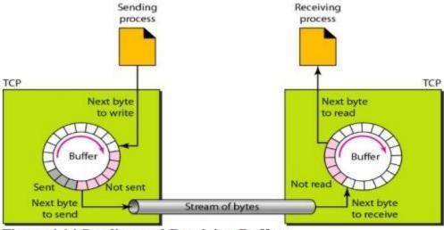
Figure 4.14 Sending and Receiving Buffers
