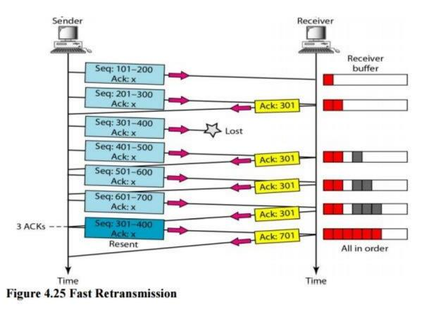
When the receiver receives the fourth, fifth, and sixth segments, it triggers an acknowledgment. The sender receives four acknowledgments with the same value (three duplicates). Although the timer for segment 3 has not matured yet, the fast transmission requires that segment 3, the segment that is expected by all these acknowledgments, be resent immediately.
