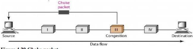
Figure 4.29 Choke packet
