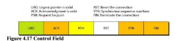
These bits enable flow control, connection establishment and termination, connection abortion, and the mode of data transfer in TCP. A brief description of each bit is shown in Table 4.3
