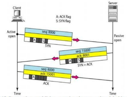
Figure 4.18 Connection establishment using three-way handshaking
