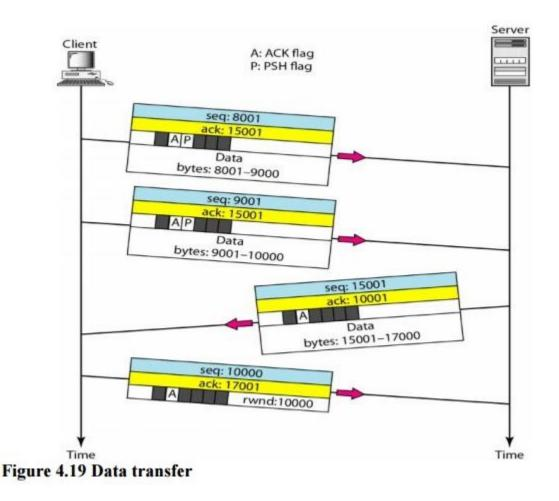
TCP can handle such a situation. The application program at the sending site can request a push operation. This means that the sending TCP must not wait for the window to be filled. It must create a segment and send it immediately. The sending TCP must also set the push bit (PSH) to let the receiving TCP know that the segment includes data that must be delivered to the receiving application program as soon as possible and not to wait for more data to come.
