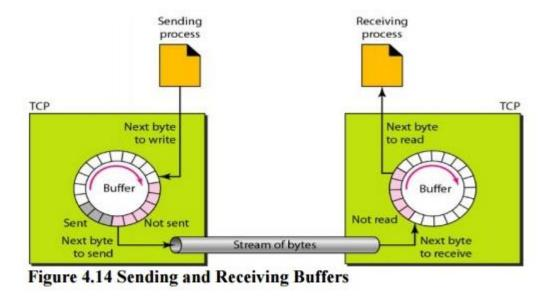
Figure 4.14 shows the movement of the data in one direction. At the sending site, the buffer has three types of chambers. The white section contains empty chambers that can be filled by the sending process (producer). The gray area holds bytes that have been sent but not yet acknowledged. TCP keeps these bytes in the buffer until it receives an acknowledgment. The colored area contains bytes to be sent by the sending TCP.
