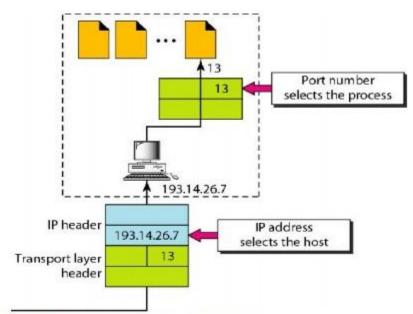
Figure 4.3 IP addresses versus port numbers
